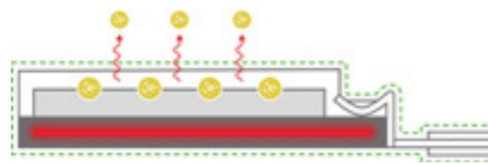
**Automatic Sensor ReCovery (ARC) for chemical contamination:** This function ensures long-term stable measurements, even under chemical contamination. During regeneration, the sensing element is heated intensely to remove deposits and effectively prevent potential measurement drift.
