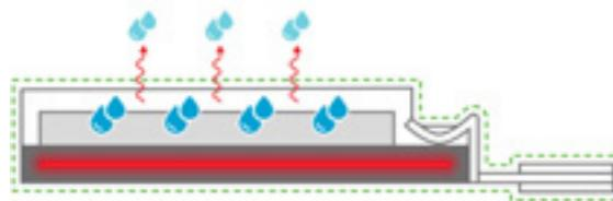
**Integrated sensor heating (High Humidity Guard):** By continuously, precisely heating the sensing element and the probe body, condensation is effectively prevented in applications with permanently high humidity. This extends sensor service life and long-term stability while reducing maintenance requirements.
