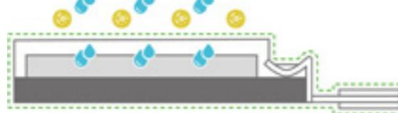
**E+E Sensor-Coating:** Developed by E+E Elektronik, this proprietary protective layer is applied to the active surface of the sensing element. It extends the sensor's lifetime and further improves long-term stability in demanding, dusty or contaminated environments.
