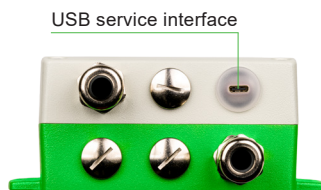
Fig. 19 USB service interface
