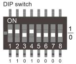
Modbus address setting via DIP switch:
