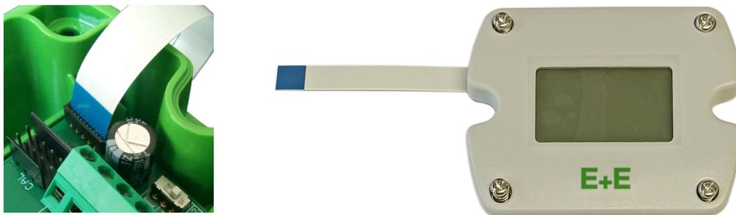
Fig. 4 Display and FFC cable connection on the EE211 electronics board
