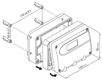
Fig. 6 Mounting of polycarbonat enclosure
