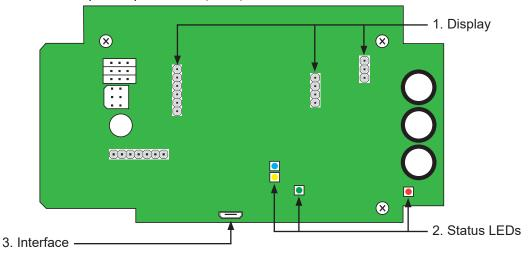
Fig. 3 Electronics board model T5
