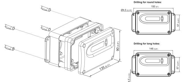
Fig. 5 Mounting of metal enclosure
