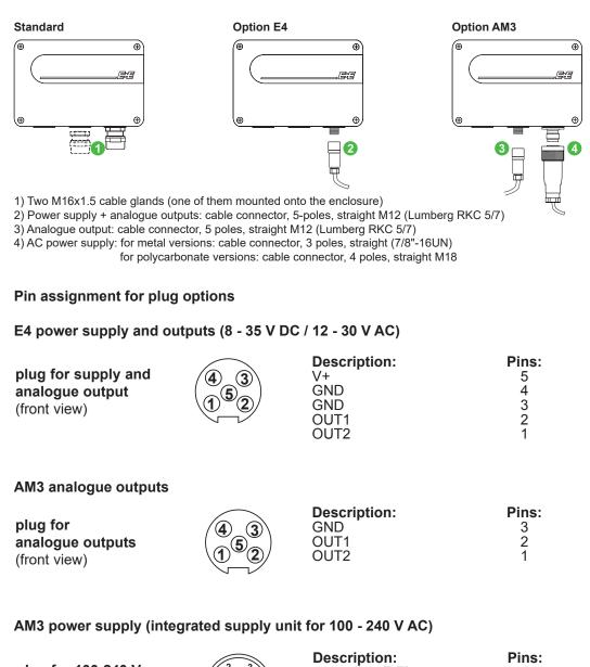
plug for 100-240 V grounding (PE) 1 metal enclosure phase (L1) 2 neutral wire (N) 3 (front view) **Description:** Pins: plug for 100-240 V phase (L1) 1 3 polycarbonate enclosure neutral wire (N)
