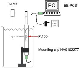
Fig. 6 Temperature calibration/adjustment in a liquid bath
