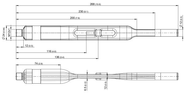
Fig. 1 Dimensions of EE260 in mm (inch)
