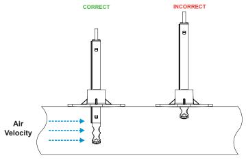
If the sensor probe is installed without a mounting flange, ensure that the air velocity sensor is aligned parallel to the air stream.
