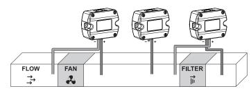
Use a Ø7.5 mm drill to install the pressure connection nipples into the duct.
