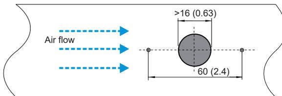
The arrow engraved on the sensing head of EE650 indicates the direction of the air stream during factory adjustment.
