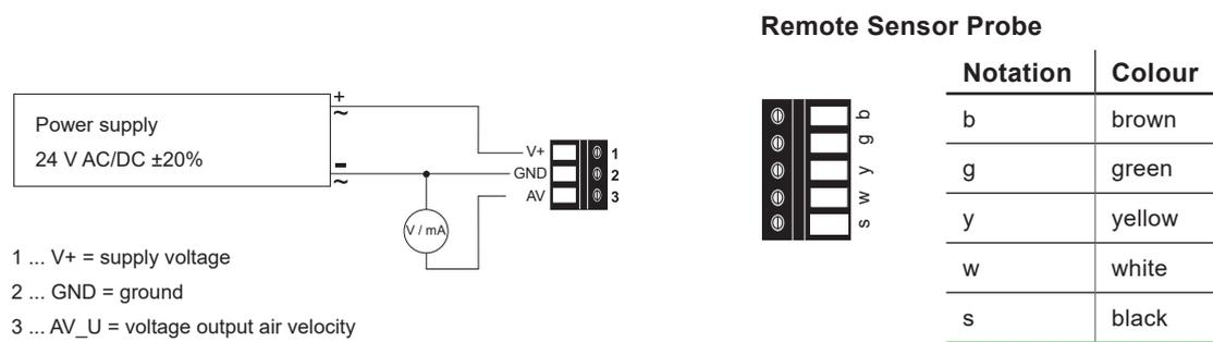
Fig. 1 Connection diagram for analogue output
