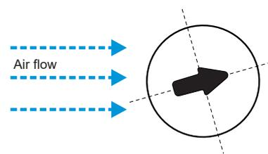
The mounting flange allows for precise setting of the EE650 immersion depth in a duct. The entire sensing head must be in the air flow to be measured.
