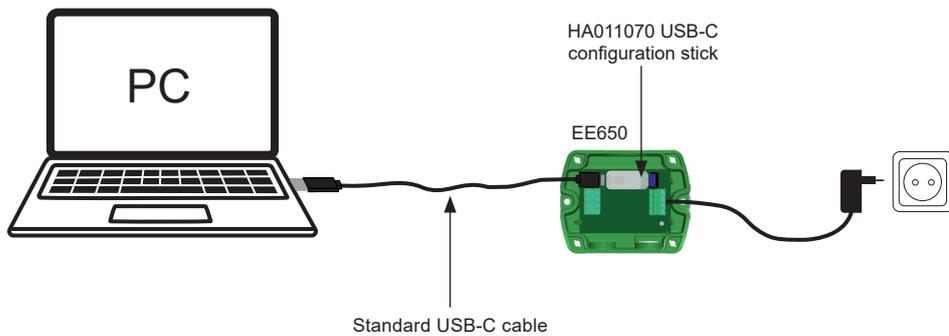
Fig. 3 EE650 configuration using the HA011070 USB-C configuration stick
