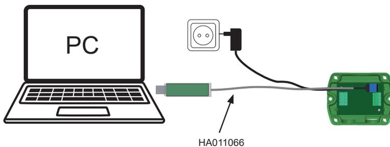
Fig. 4 EE650 connected to a PC running PCS10
