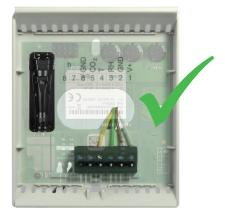
EE800 features a protection cap for the CO<sub>2</sub> sensing cell. Although this facilitates the handling during installation and diminishes the chances of unintended mechanical impact onto the cell, please observe the wiring guidelines as above. Do not attempt to remove the protection cap.
