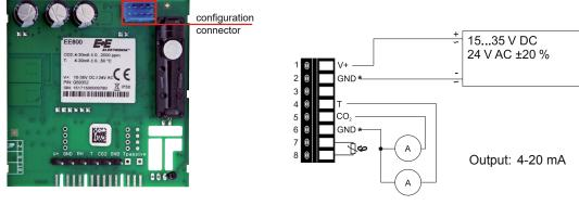
\* Very important: for failure-free operation and performance according to the specs the supply GND and the measurement GND must be wired separately.
